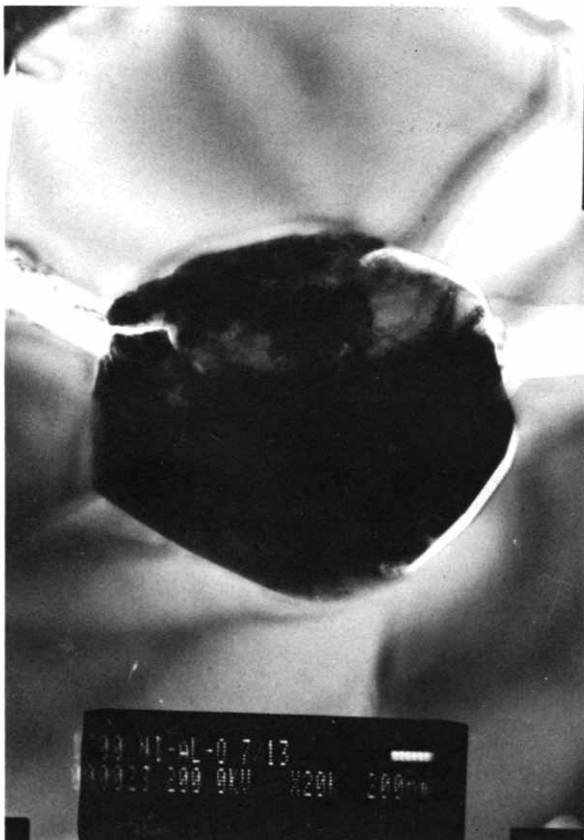
Fig. 5. Bridging nickel particle observed in the composite prepared by the gas reduction process. Note the debonding at the interface.
